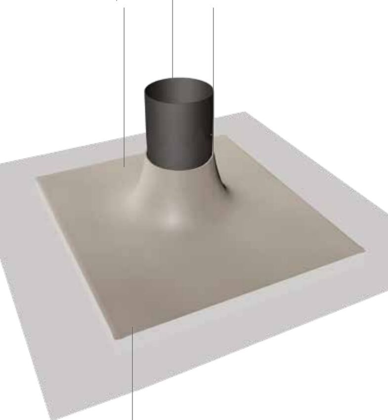
CrysticROOF® Topcoat over GRP resin layer
