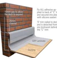
Fix ALL adhesive ap-plied to back of "C" trim and secured into place
