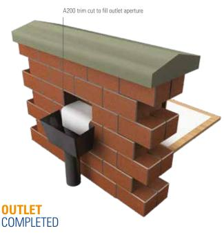
To allow water to flow into the gutter an 'A' type drip trim should be used. In order to allow the drip trims to sit level with the roof and to prevent water from ponding in the outlet, the board forming the outlet should be rebated by 3mm.
