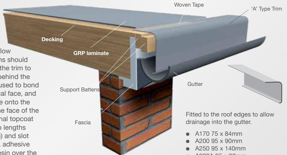
Fitted to the roof edges to allow drainage into the gutter.
